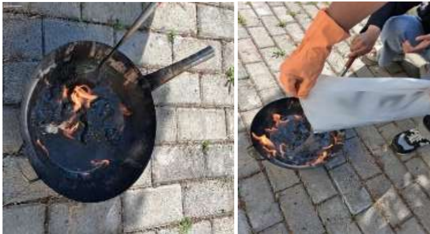
Figure 2. Melting process of LDPE plastic waste and Mixing molten LDPE with sand
