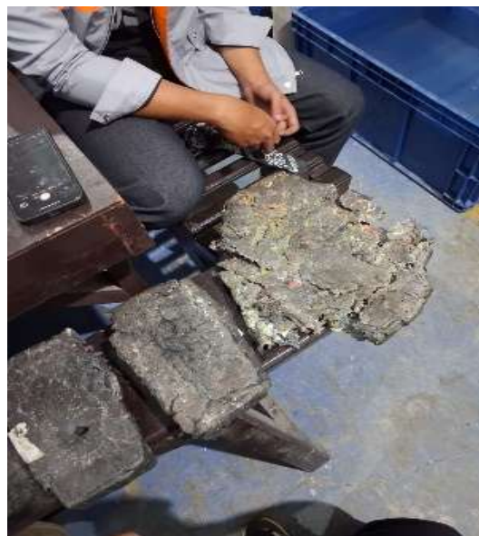
Figure 6. Failure pattern after compressive strenght test
