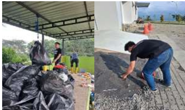
Figure 1. LDPE plastic waste and natural sand used as raw materials
