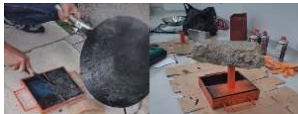
Figure 3. Casting and compaction process.
