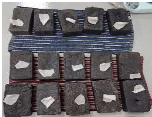
Figure 4. EcoPlast Paving Blocks with three different mix compositions
