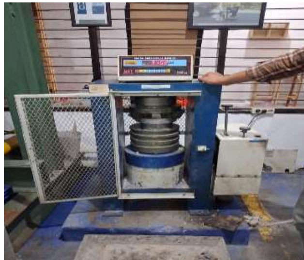
Figure 5. Compressive strenght testing using a Universal Testing Machine (UTM)
