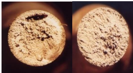
(a) quench 840°C (b) quench 840°C, temper 200°C
