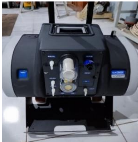
Figure 4. Gas analyzer, a tool for measuring exhaust emissions
