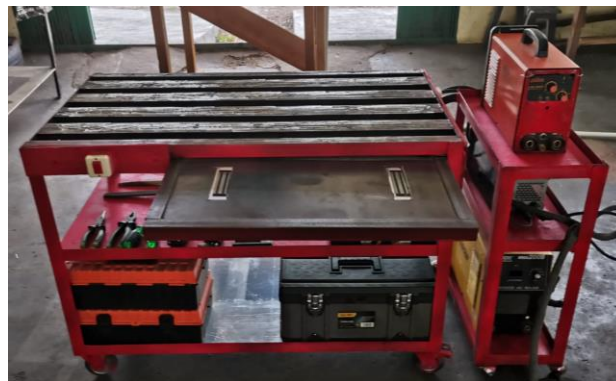
Figure 4. Electromagnetic Welding Table Prototype
