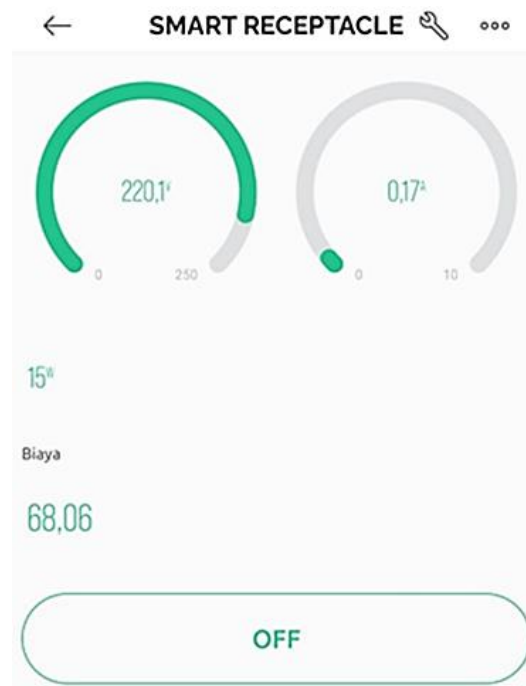
Figure 7. The interface of the Smart Receptacle Application on Blynk
