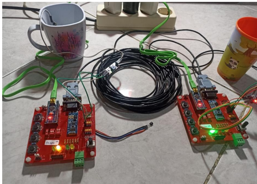
Figure 7. Slave distance testing with master slave architecture
