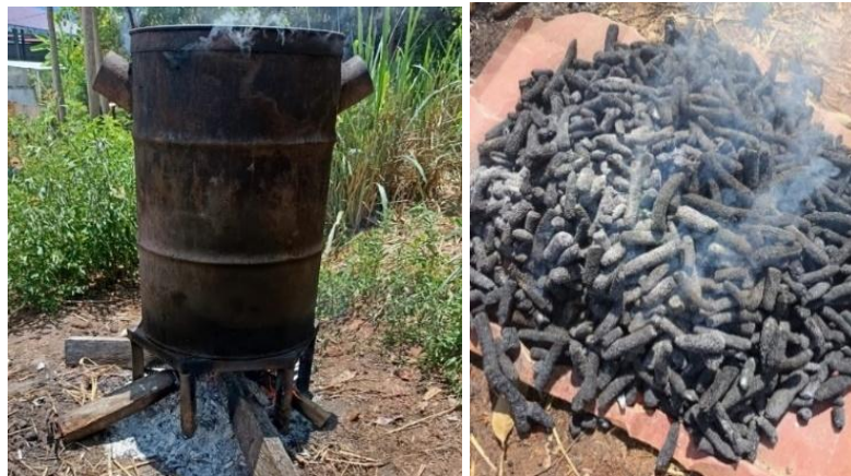
Figure 2. Charcoal Making Process
