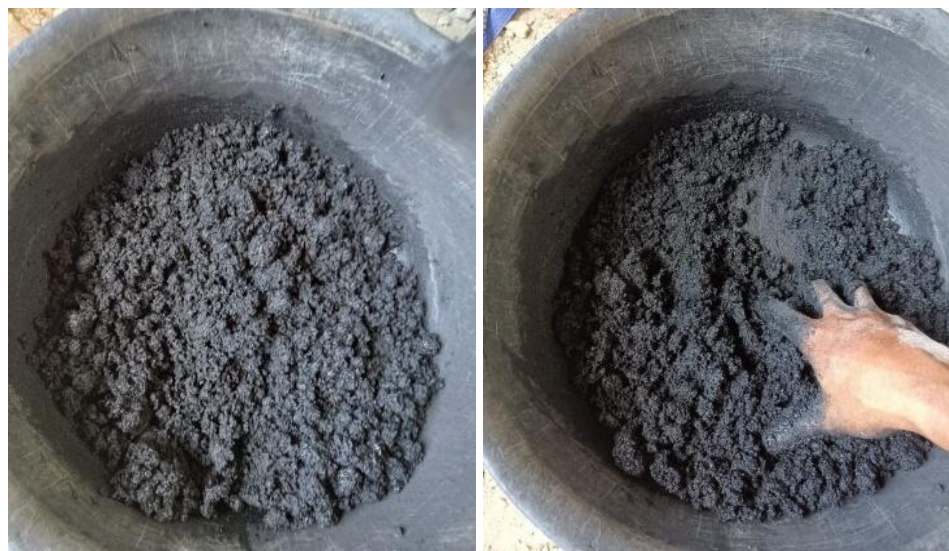
Figure 3. Process of mixing charcoal powder with adhesive
