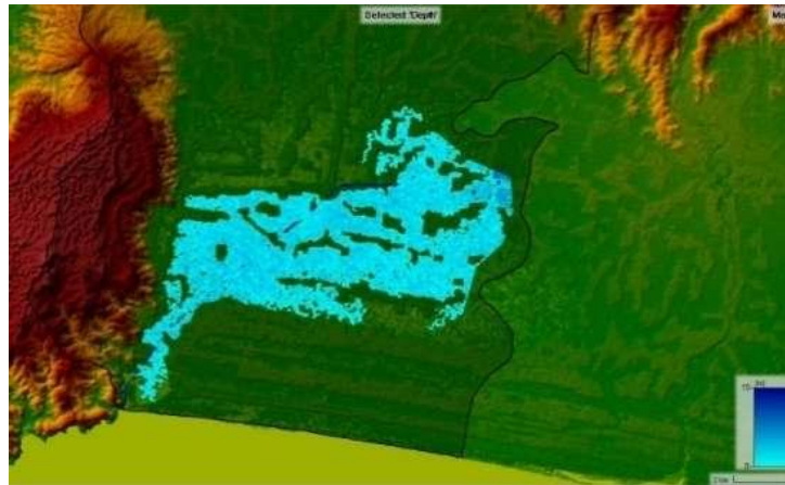
Figure 6. Results of Flood Modelling using HEC-RAS 6.4.1
