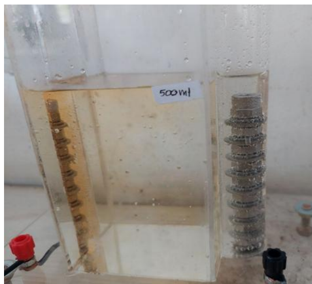
Figure 4. Results of Hydrogen Gas Bubble Test
