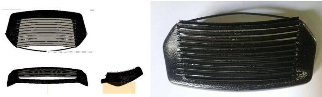
Figure 5. (a) Design of speedometer cover (b) Result of 3D Printing
