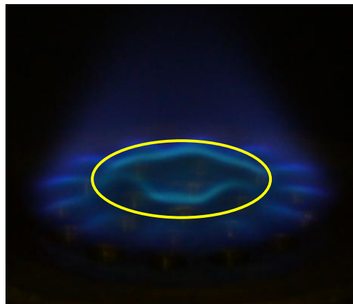
Figure 4. Morphology of cellular flame structure (cells flame)
