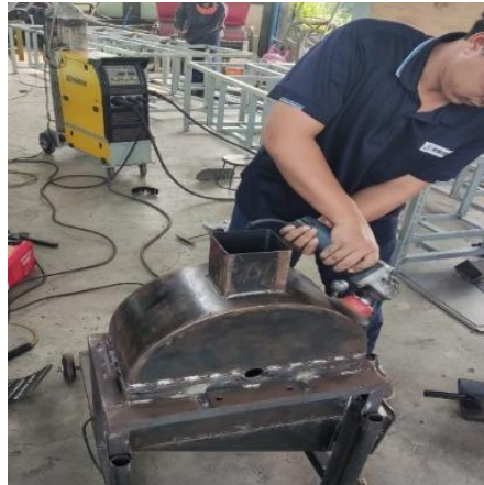
Figure 3. Welding Process for Making Shredding Machine Frame
