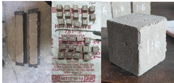
Figure 3. Test cube specimens measuring 50 × 50 × 50 mm
