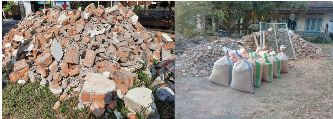
Figure 1. The material used in this study consists of rubble from demolished building walls in the Yogyakarta region
