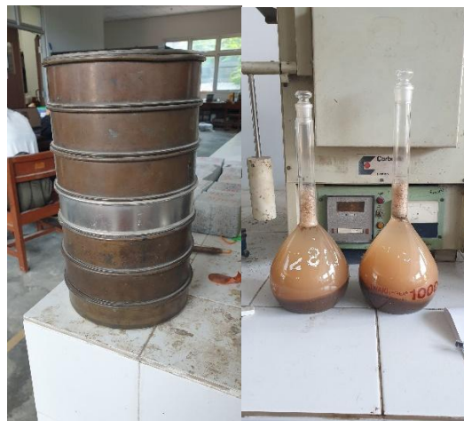
Figure 2. The gradation and specific gravity tests were conducted on recycled rubble obtained from the demolition of wall structures.
