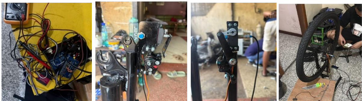
Figure 5. Assembling the arduino box, electronic components, and the servo arm with the brake caliper arm.
