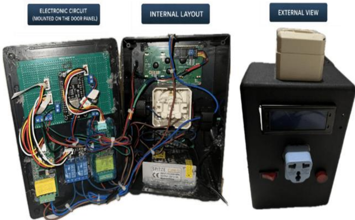
Figure 6. Implementation of the Smart Energy Meter System
