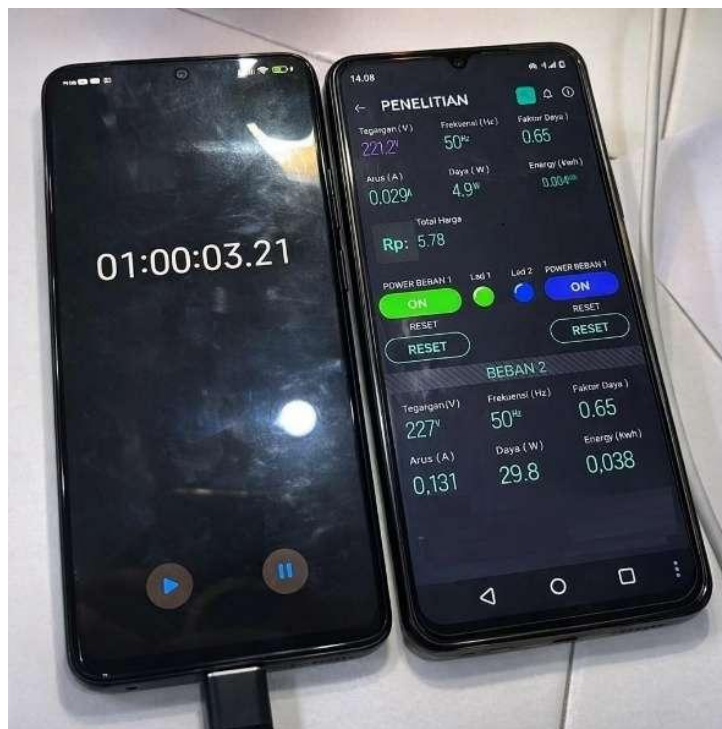
Figure 8. Real-Time Monitoring Interface of the Smart Energy Meter System
