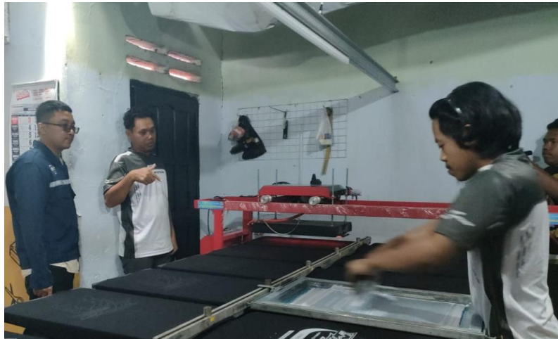
Gambar 4. Kegiatan uji coba flash curing gas autoslide
