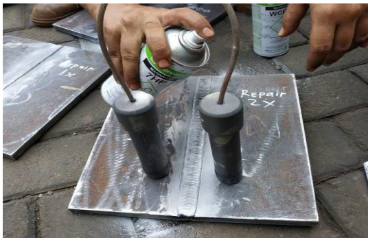
Gambar 12 Proses magnetizing test pengelasan repair 2x
