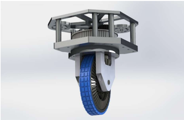
Gambar 1. Desain 3D modular Swerve drive
